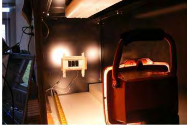
Figure 11. Photograph of the indoor solar panel testing set-up
